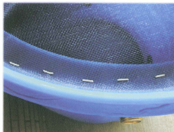
Figure 6. Cut excess screen with utility knife or scissors.
