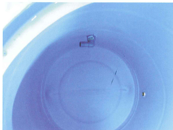
Figure 4. Screw the elbow onto the adaptor for added support. (multiple barrel only)
