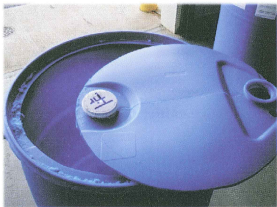
Figure 1. Cut top of barrel at least 1" from edge.
